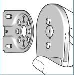
Push the pin of the clutch and take the clutch out of the bracket.
