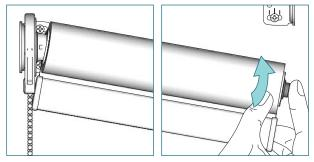
Insert the tube on to the clutch head. Press the tube bearing plug and lift the shade.
