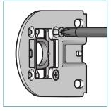
Make sure that the opening for the Allen key is pointing downwards before installing the brackets. Change the orientation by removing the 2 screws and turning the leveler 90°. Reinstall the screws.
