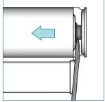
Slide the bracket cover towards you. Place a screw driver between the tube bearing plug and bracket and push the bearing in the clutch direction.
