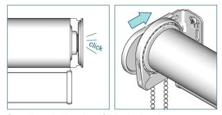
Snap it to the bracket. Slide the bracket covers on to the brackets.
