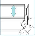
To adjust skewing, put the provided Allen key into the screw of the leveler and turn it left or right to move the shade up or down. Support lifting of large heavy shades with the palm of your hand.
