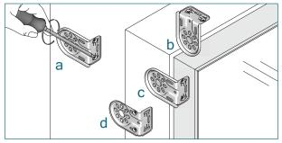
Install the brackets with the screws provided.
