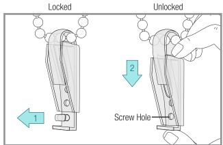
To unlock, remove the plug from the screw hole and push down.
