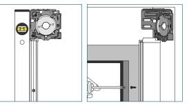
Level the side guiding channel flush with the backside of the bracket. Fix the channel in this position (with provided screws).
