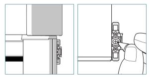
Place the side guiding channel sidewise into the upper clip. Level the side guiding channel. Slide a clip to the lower position. Level the bottom of the clip and side guiding channel.
