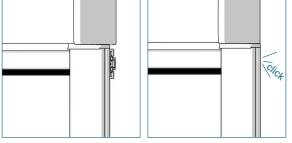
Place the side guiding channel above the clips. Snap the channel into the clips. Fix the left side guiding channel just like the first channel.
