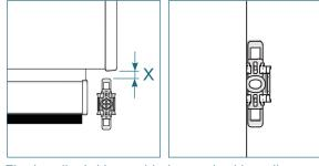
Fix the clip (with provided screw) with a distance X = 5 mm to the bottom of the end cap. Snap the other clips sidewise onto the side guiding channel.
