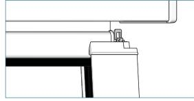
Unclip the side guiding channel. Place the bottom rail into the side guiding channel.
