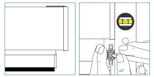
Install the roller shade. Level the clip flush with the end cap. Mark the horizontal position of the screw.
