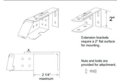
**Hold-Down Brackets:** Use hold-down brackets to prevent blinds from swaying when mounted on doors or exposed to the wind. Screw hold-down bracket into the lower corner of window jam or sill. Drill a small hole in the center of the bottom rail to slip hold-down pin (extending from hold-down bracket) into blind.
