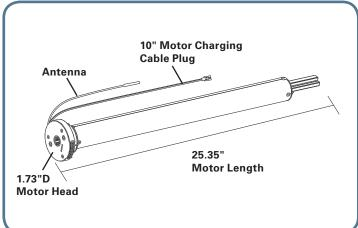
FOR OPTIMAL PERFORMANCE, THE ANTENNA WIRE MUST BE EXPOSED AND NOT COME IN CONTACT WITH METAL SURFACES. DO NOT CUT ANTENNA WIRE. REPOSITION AS NECESSARY.
