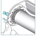
Fit the motor front plate into the motor bracket.
