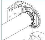
Insert the provided Allen key into the set screw of the leveler.
