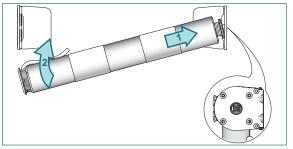
Place the roller shade end plug into the idle end bracket. Push the shade against the idle end and lift the motor end up.
