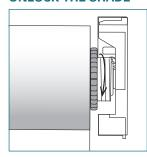
Rotate the nut on the idle end counterclockwise to unlock the shade.
