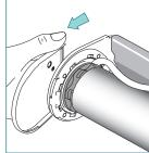
Lift the backside of the endcap away from the bracket, then slide the end cap towards you.
