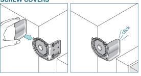
Slide the screw cover cap onto the bracket until it snaps.
