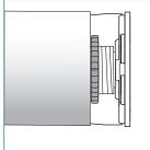
Rotate the nut on the idle end clockwise until it meets the tube. This locks the shade into position.
