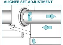
To align the bottom hembars, pull the shade away from the aligner set (1), turn the shade to line up the bottom hembars together (2). Release the shade to secure the position (3). Not possible when using a connector set.
