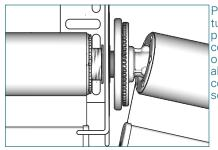
Place the tube with plug connector on the aligner or connector set head.
