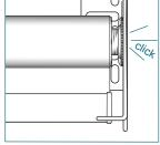
Press the tube bearing plug, lift the roller shade and snap into the idle bracket end.
