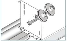
Slide the aligner or the connector through the bracket into the idle end.
