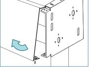
Remove the screw. nut, and washers.
