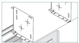
Fix the outer bracket with the screws provided.
