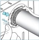
Turn the roller shade approximately 10° in the rolling direction and close both fasteners of the brackets.
