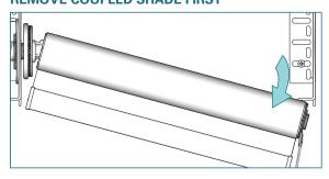
Place a screwdriver between the bracket and bearing plug and push towards the aligner to remove the shade. Move the shade downward and out of the bracket. Remove the aligner or connector from the bearing plug.
