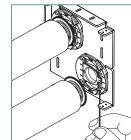
Insert the provided Allen key into the set screw of the leveler.
