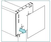
Peel the end plate from the bracket. Use a flat head screw driver to pry off if necessary.
