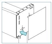
Remove tape from end plate and attach to bracket.
