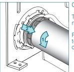
Open the bracket fasteners.
