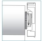
Rotate the nut on the idle end counterclockwise to unlock the shade.
