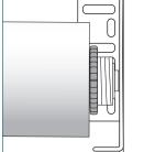
Rotate the nut on the idle end clockwise until it meets the tube. This locks the shade into position.
