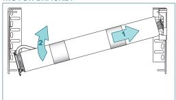
Push the shade against the idle end and lift the roller shade up until the motor front plate fits into the motor bracket.
