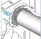
Turn the roller shade approximately 10° in the rolling direction and close both fasteners of the brackets.
