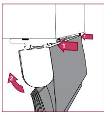
Angle the shade so that the front ridge of the headrail can rest on the front teeth of the bracket.
