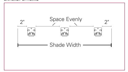
Mount into wood or metal studs or into concrete with concrete anchors. Drywall anchors are not recommended.
