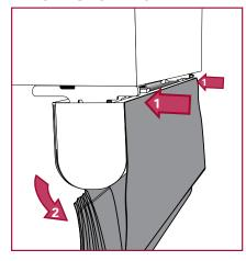
Securely hold the headrail. Push the headrail towards the back of the shade and tilt the back of the shade down until the headrail releases from the back teeth of the bracket. Move the headrail towards the front of the shade to remove completely from the brackets.
