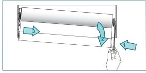
Slide a flat head screwdriver between the idle end plug and bracket and push towards the clutch end to remove the plug from the bracket.
