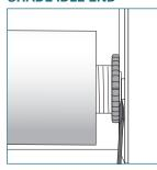
Slide a flat head screwdriver between the idle end plug and bracket and push towards the clutch end to remove the plug from the bracket.
