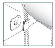
Thread the chain out of the chain guide.
