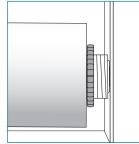
Rotate the nut on the idle end clocwise until it meets the tube.
