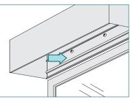
Mount into wood or metal studs or into concrete with concrete anchors. Drywall anchors are not recommended.
