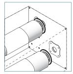
Install the front shade. Place the clutch onto the clutch bracket.
