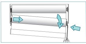
Move the shade downward and out of the clutch bracket.
