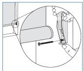
Be sure the cord tensioner(s) is not placed in the path of the bottom rail and fabric.
