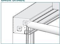
Install the back shade first. Place the clutch onto the clutch bracket.
