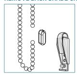
Remove the chain connector from both sides of the chain.
