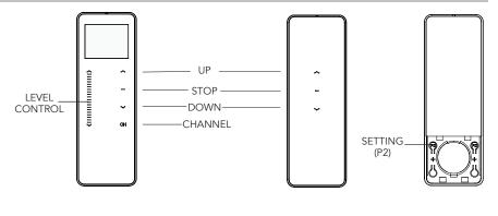
Remove cover from remote press gently in and down to disengage cover.
