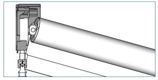
Place the tube adapter on the crank head.
