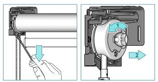
Place the screw driver into the slot of the locking clip. Press the locking clip down and turn the crank in the roll-up direction. Take the crank out of the bracket.
