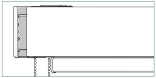
Slide the bracket covers onto the brackets.
