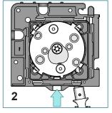
Insert the crank with the front plate into the bracket (1). Turn the crank in the rolling off direction and secure it with the locking clip (2).
