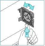
Insert the Plate L into the bracket on the nonoperating side. Turn the Plate L in the rolling off direction (1) and secure it with the locking clip (2). Not necessary when using bracket with leveler.
