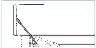
Place the screw driver under the bracket cover, turn the screw driver and slide the bracket cover from the bracket.
