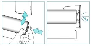
Press the tube bearing plug (1), lift the shade and snap into the bracket.
