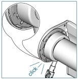
Slide the bracket covers onto the brackets. Make sure the bracket covers snap onto the brackets.
