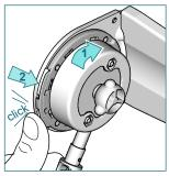
Slide the crank into the bracket adapter, turn it (10°) in the rolling off direction (1). Close fastener to secure the crank.(2)
