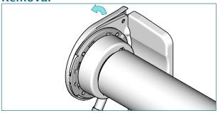
Lift the backside of the bracket cover ...
