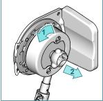
Open the fastener of the bracket adapter. Turn the crank in the roll up direction until the crank can be pulled out of the bracket adapter.
