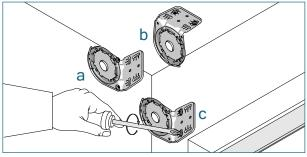
Install the brackets with the screws provided.
