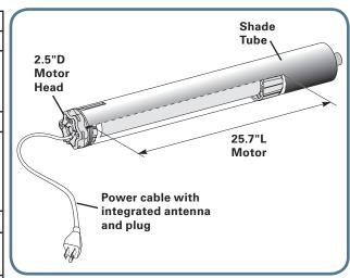
FOR OPTIMAL PERFORMANCE, THE POWER CABLE/ANTENNA MUST BE AT LEAST 18" LONG AND MUST NOT COME IN CONTACT WITH METAL.
