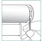
Insert the provided Allen key into the set screw of the leveler.
