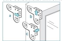
Mount into wood or metal studs or into concrete with concrete anchors. Drywall anchors are not recommended.
