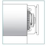
Rotate the nut on the idle end counterclockwise to unlock the shade.
