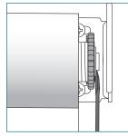
Slide a flat head screwdriver between the idle end plug and bracket and push towards the clutch end to remove the plug from the bracket.
