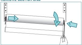
Move the shade downward and out of the clutch bracket.
