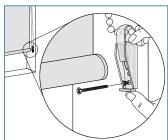
Be sure the cord tensioner is not placed in the path of the bottom rail and fabric.
