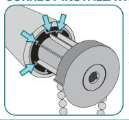
Line the ridges of the clutch up with the ridges inside the tube. Push the clutch into the tube. There will be resistance when inserting the clutch into the tube.
