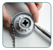
Hold the clutch by the chain guard. Rotate the clear chain wheel to make the notch accessible. Position the chain in the clear chain wheel on the opposite side of the notch. Use a screwdriver in the notch to rotate the wheel until the chain is threaded all the way through.
