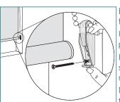
Be sure the cord tensioner is not placed in the path of the bottom rail or fabric
