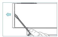
Place a flathead screwdriver under the end cap on the front of the fascia.
