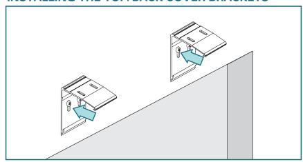
Mount into wood or metal studs or into concrete with concrete anchors. Drywall anchors are not recommended.
