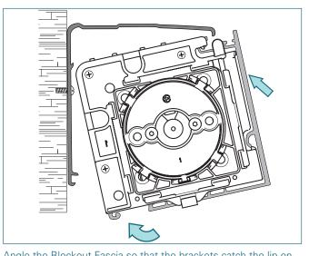
Angle the Blockout Fascia so that the brackets catch the lip on the top fascia.
